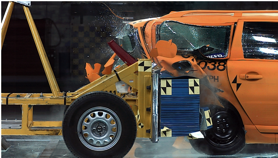
Figure 1. A destructive, rear-end collision test (Autoevolution, 2010)
